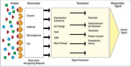
Fig 2: Biosensors and its parts.
