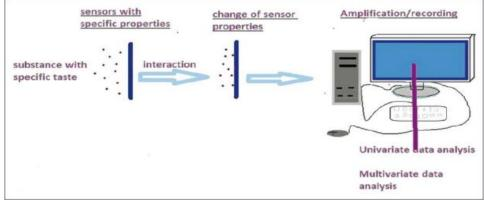
**Fig 5 :** Basic principle of electronic taste sending system[16]
