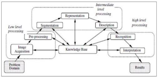
Fig 3: Different levels of image processing [6]
