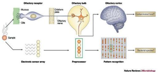
Fig. 4 : A comparison of a biological nose with e-nose [9]
